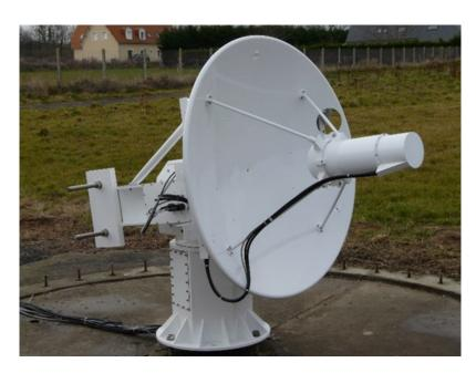
This station is designed for signals Receive in S frequency band.
